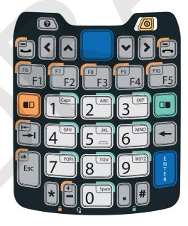
The CK70 comes with either a large alpha or an alphanumeric keypad. The CK71 comes with either a numeric function keypad or an alphanumeric keypad. The computer has an ambient light sensor that detects low light and turns on the keypad backlight. By default, the keypad backlight is enabled in low light conditions. You can disable the keypad backlight to conserve power. Use Intermec Settings to configure the backlight. For help, see "Using Intermec Settings on the Computer" on page 64.
