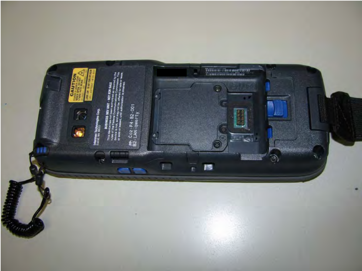
Back side – battery cover removed
