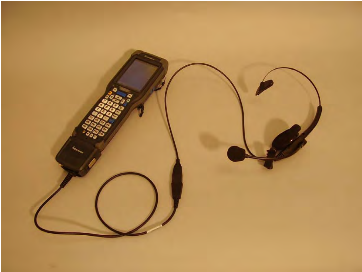
EUT with audio snap-on accessory and headset
