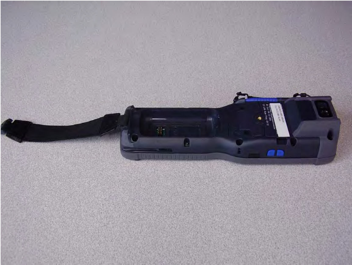
Back side – battery cover removed
