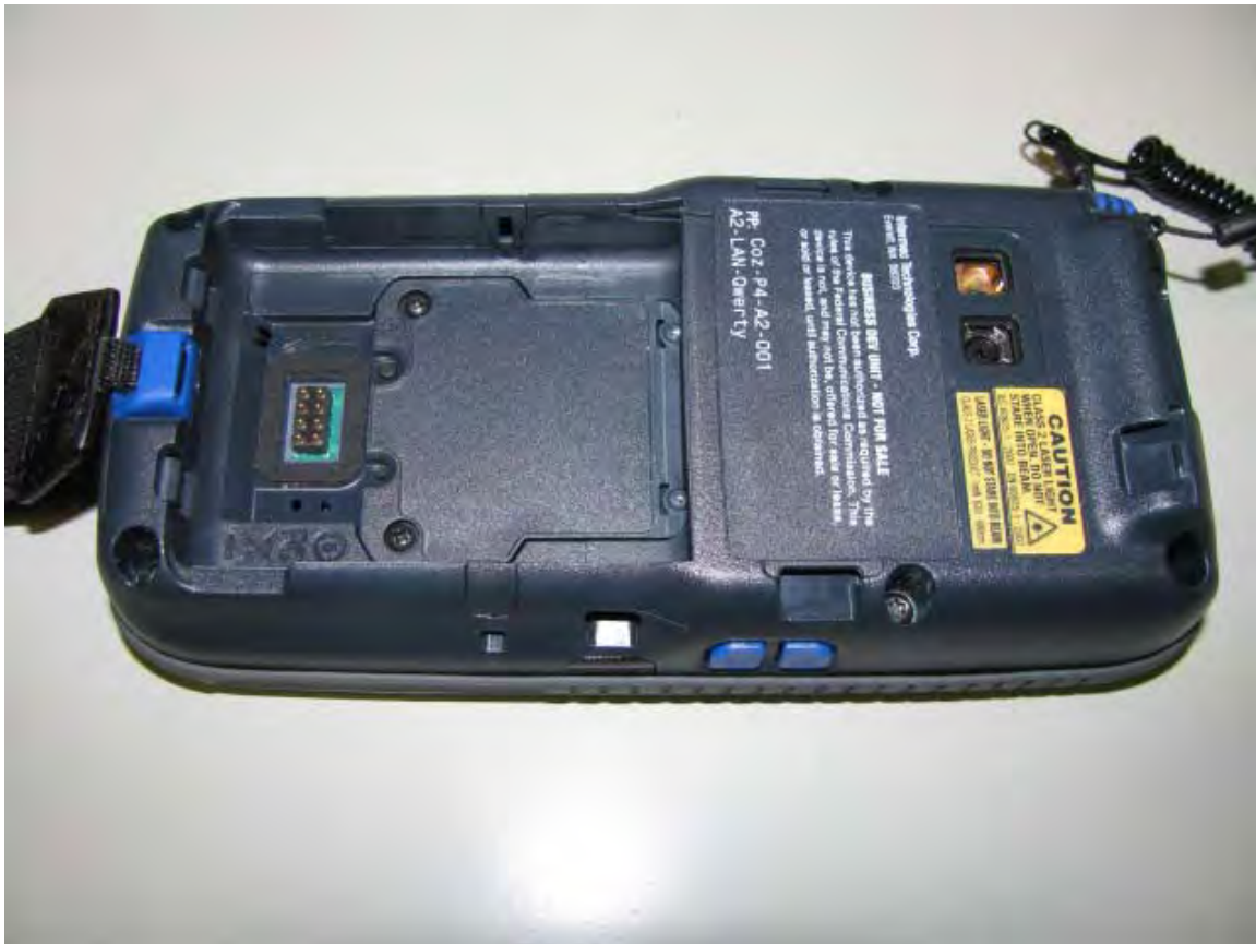
Back side – battery cover removed
