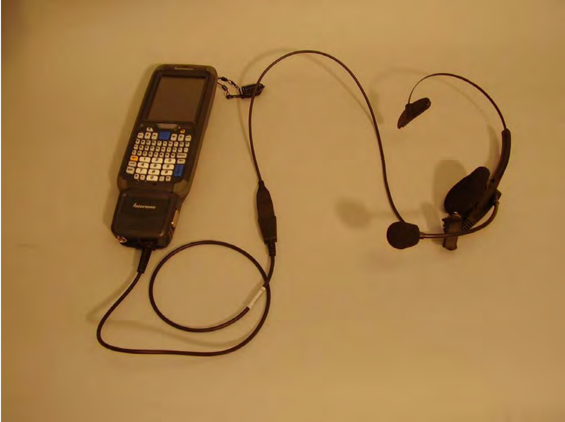
EUT with audio snap-on accessory and headset
