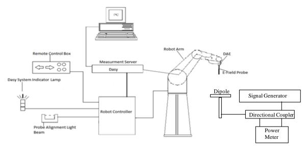
The Dasy5 HAC test system consists of:
