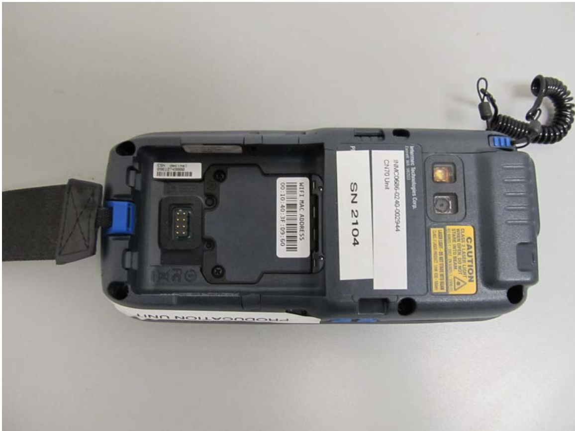
Back side – battery cover removed
