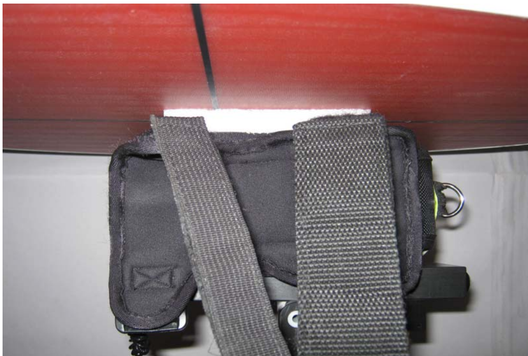
Left Side of Wrist Holster with 12mm Spacer
