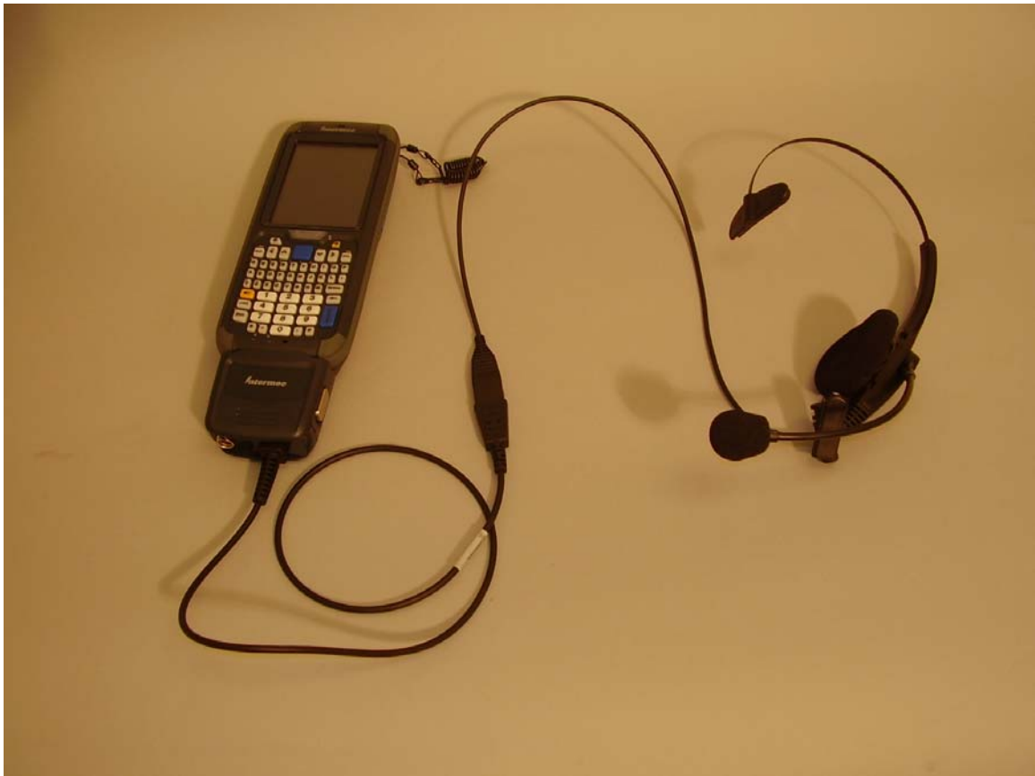
EUT with audio snap-on accessory and headset
