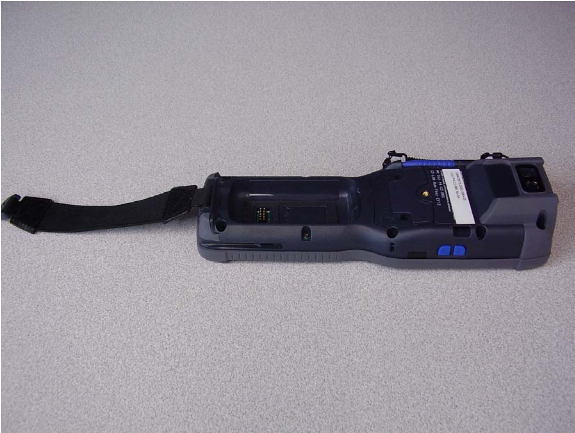
Back side – battery cover removed
