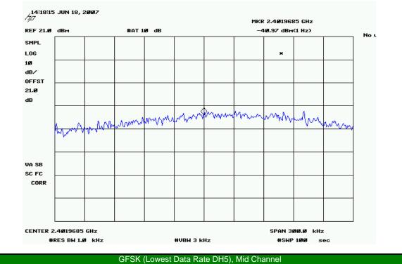
Result: Pass Value: - 6.29 dBm / 3kHz Limit: 8 dBm / 3kHz
