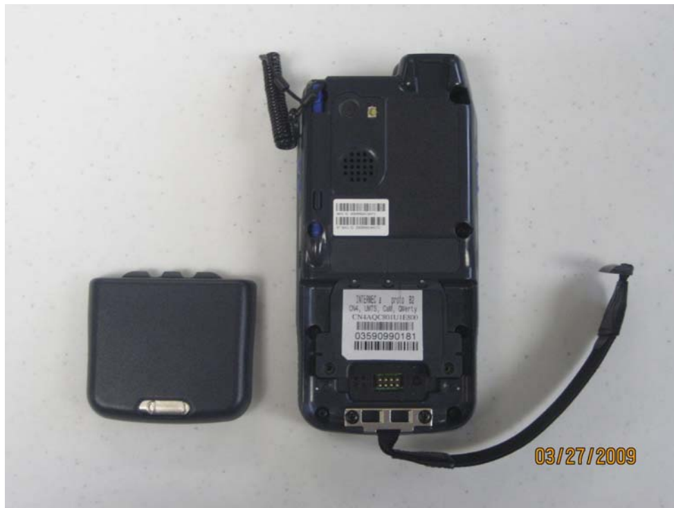
CN4_Rear View_Battery Uninstalled
