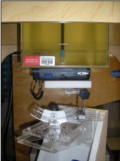
Figure 46. Positional photograph of the Interdec CN3 0.0mm front facing position.
