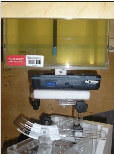
Figure 48. Positional photograph of the Interdec CN3 15.0mm front facing position.
