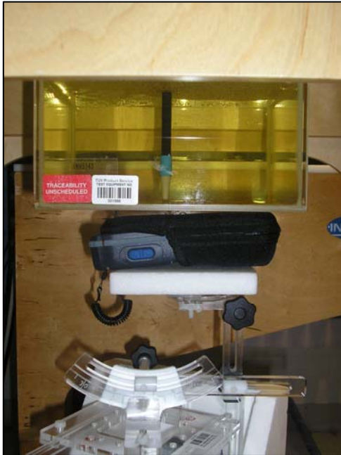
Figure 50. Positional photograph of the Intermec CN3 0.0mm front facing position in holster.
