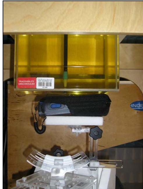
Figure 51. Positional photograph of the Intermec CN3 0.0mm rear facing position in holster.
