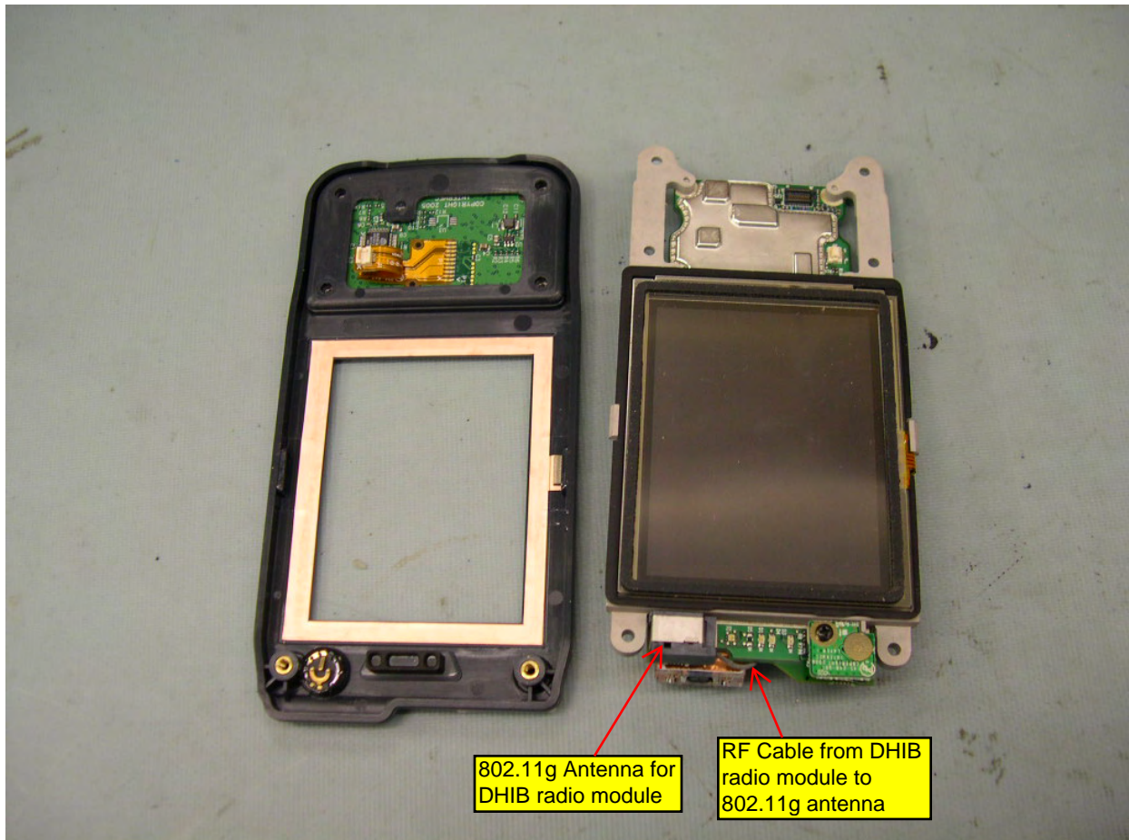
CN3 Unit with main PCB removed from front housing to show 802.11g antenna
