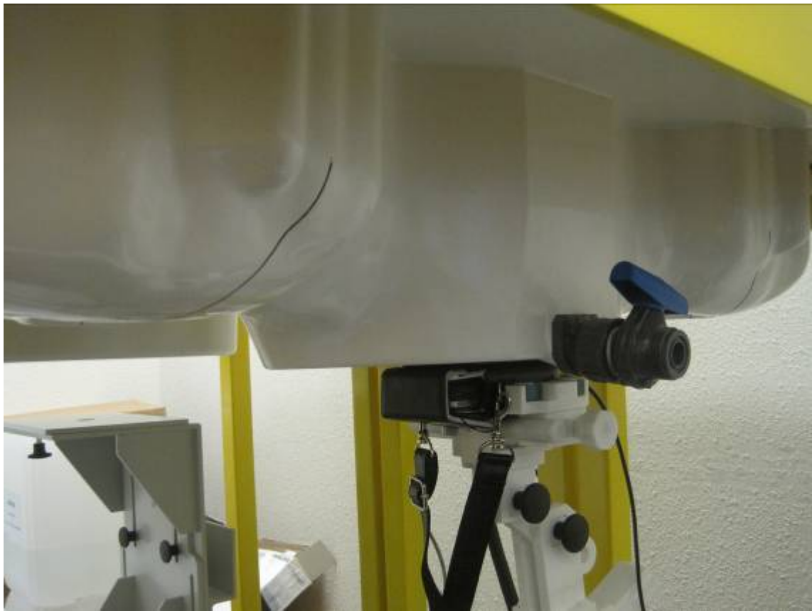
Body SAR test setup with purse -3
