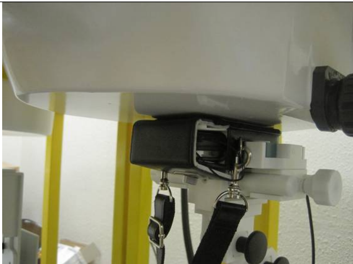
Body SAR test setup with purse -1
