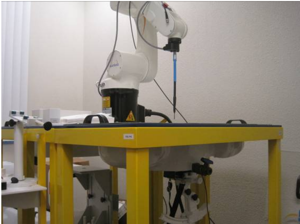
Body SAR test setup with purse -4
