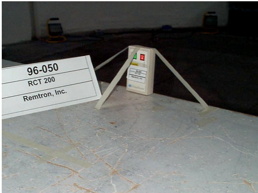
*3.1.7 Photograph of Radiated Test Setup – Rear View - per 2.1033(b)(7)*
