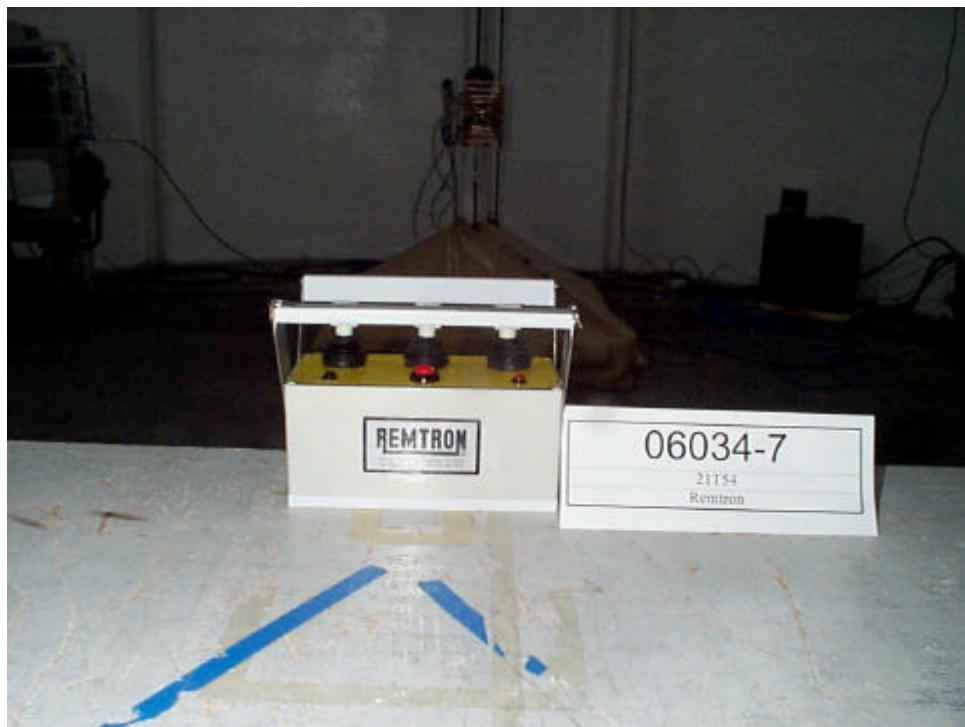
Belly Box Transmitter 21T54 (903.0 MHz to 927.0 MHz) PCB
