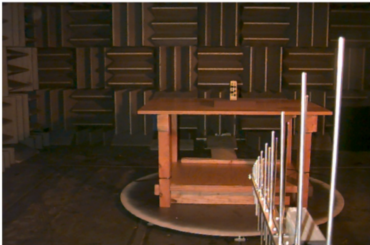
Radiated Emissions, Fundamental Vertical Polarization EUT in position 2
