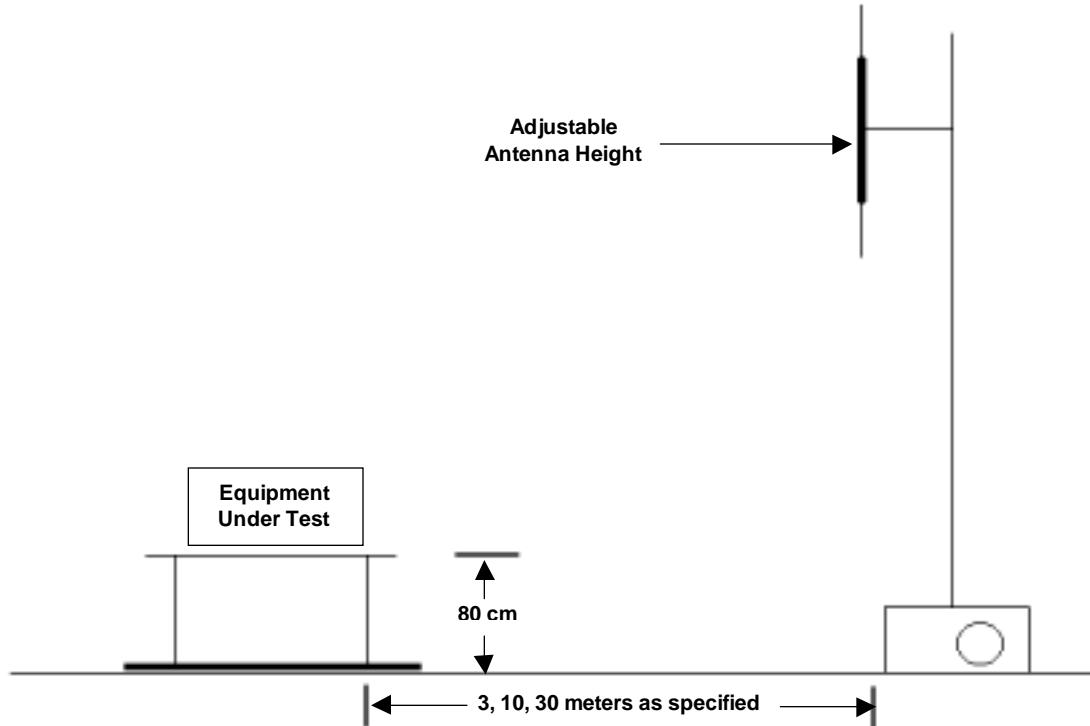
**Radiated Test Setup and Procedure - cont'd**
