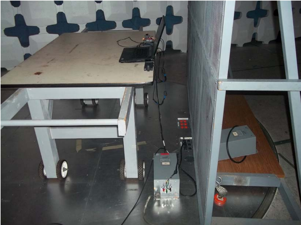
Conducted Emissions Test Configuration Photograph
