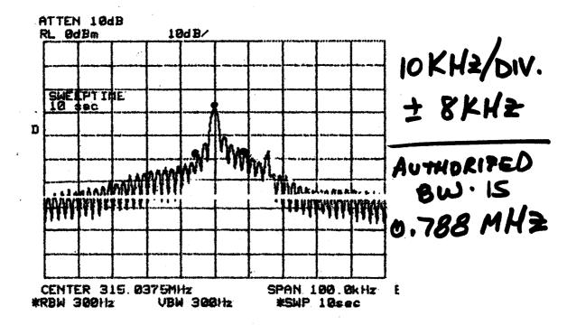
**DEVICE: DXS-65 Remote Control Transmitter**
