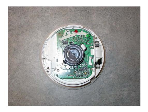
DXS-73 INTERIOR VIEW, TRANSMITTER PCB ATTACHED TO MAIN PCB VIA 4 PIN CONNECTOR
