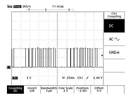
17 BITS / DATA WORD + 3 BLANK FRAMES BETWEEN WORDS DATA WORD = 20 X 5000 USEC = 100 MILLISECONDS FOR NOMINAL DATA WORD FRAME
