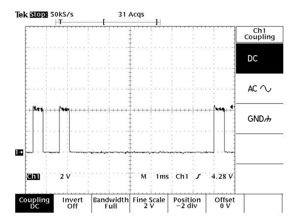
INDIVIDUAL DATA PULSES, QUATERNARY ENCODED DATA FORMAT 500 uSEC FOR EACH DATA PULSE
