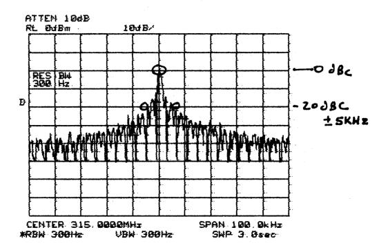
DEVICE: DXS-LRP Remote Control Transmitter
