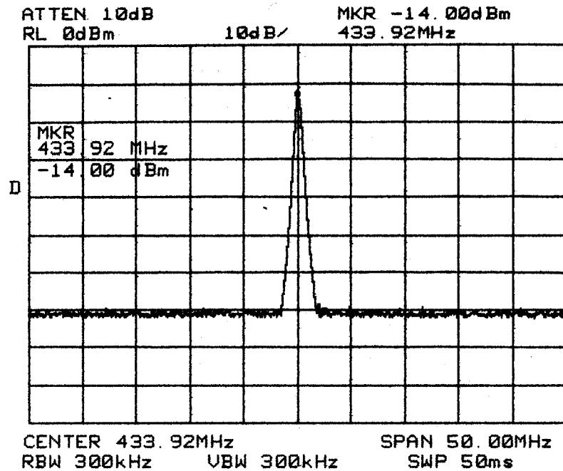
DEVICE: DXS14 Remote Control Transmitter
