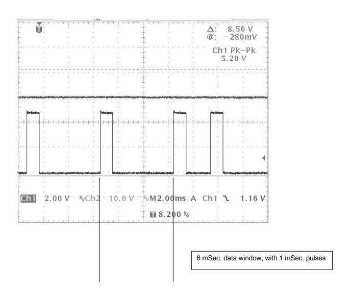
Single Data Pulses, 1 mSec. pulses in a 6 mSec. data window.
