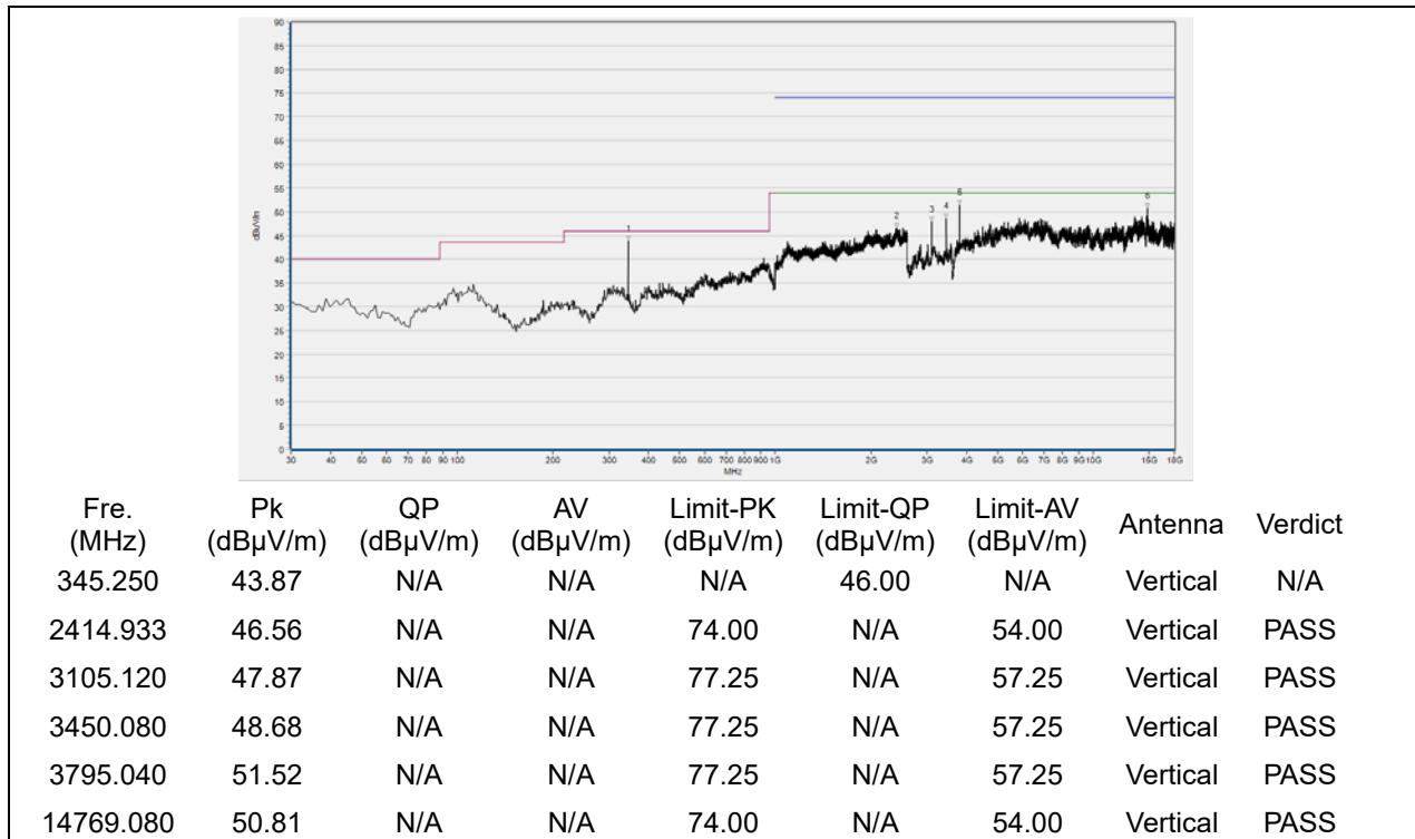
(345 MHz, Antenna Vertical, 30 MHz to 5 GHz)
