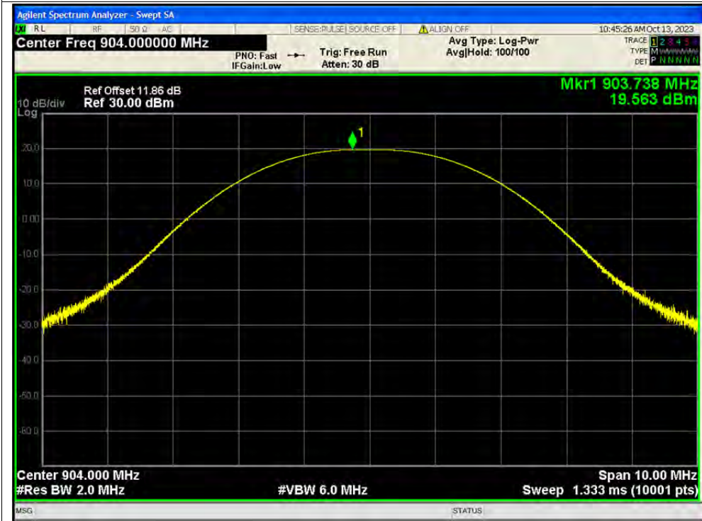
Peak Power NVNT 900M_Non-Hopping 912MHz Ant1
