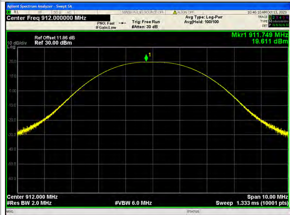
Peak Power NVNT 900M_Non-Hopping 912MHz Ant1
