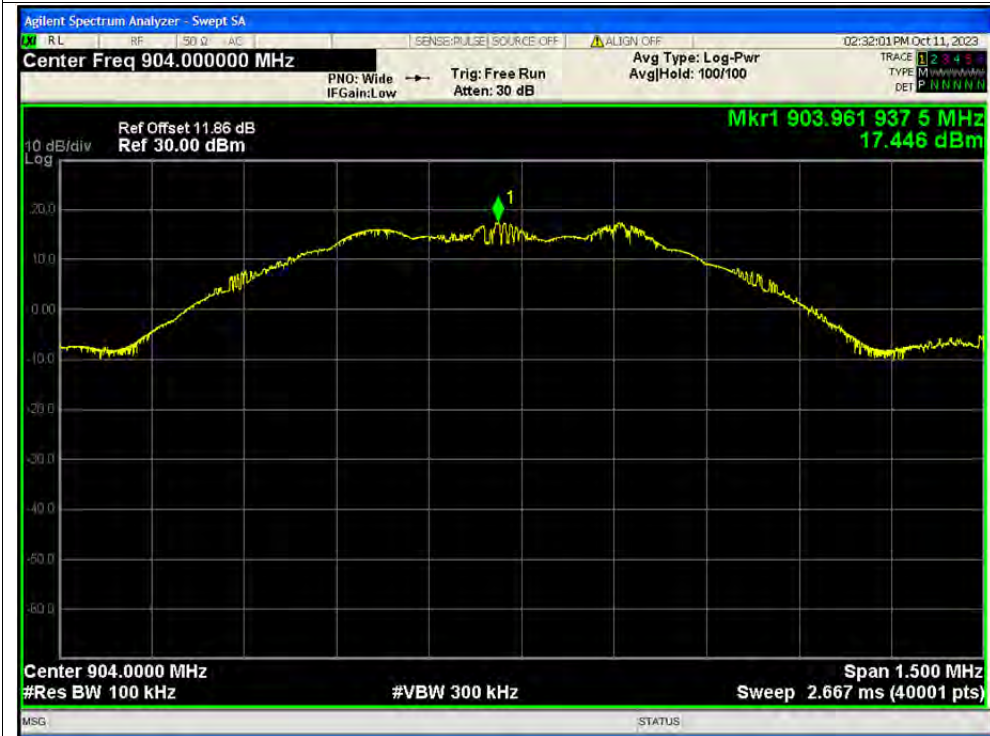
Tx. Spurious NVNT 900M_Non-Hopping 904MHz Ant1 Emission
