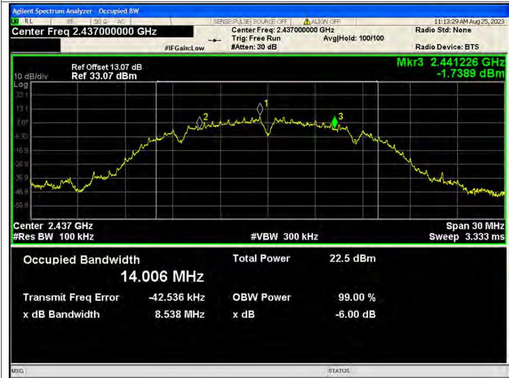
-6dB Bandwidth NVNT b 2437MHz Ant1
