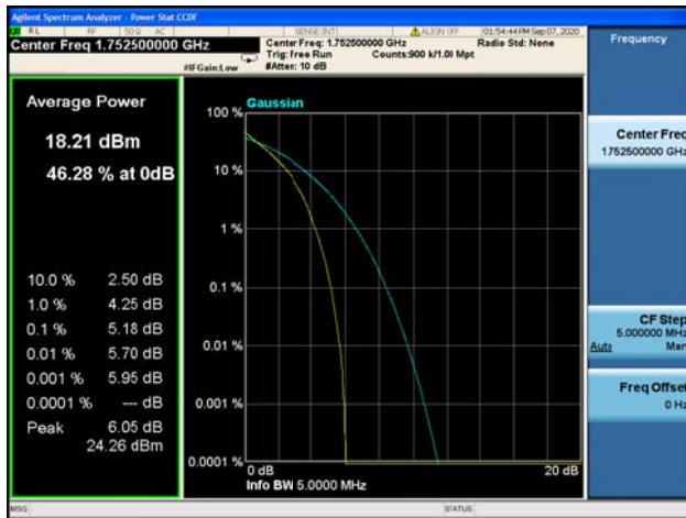
Band 4 / 5MHz / High CH / QPSK
