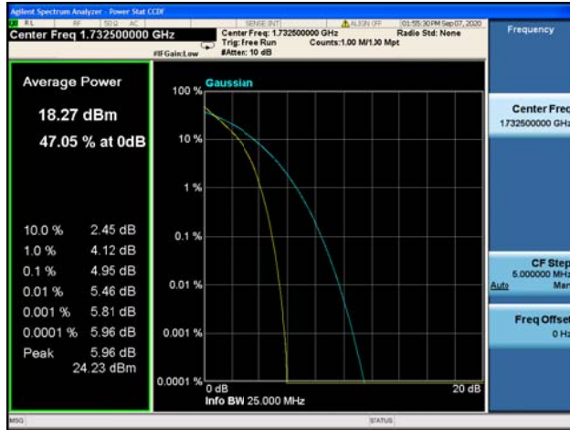
Band 4 / 15MHz / High CH / QPSK
