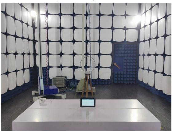
3. Radiated emission (9KHz-30MHz)
