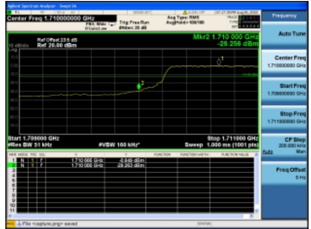
Band4 / 5MHz / High CH / QPSK / FULL RB
