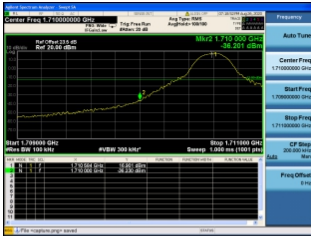
Band4 / 10MHz / High CH / QPSK / 1 RB
