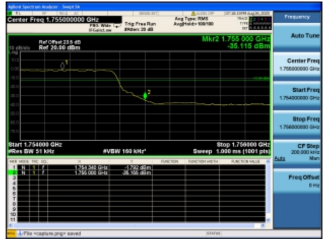
Band4 / 5MHz / High CH / QPSK / FULL RB
