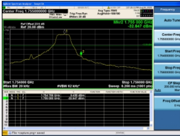
Band4 / 1.4MHz / High CH / QPSK / 1 RB
