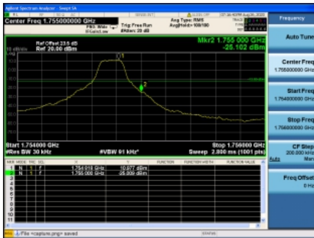
Band4 / 3MHz / High CH / QPSK / 1 RB
