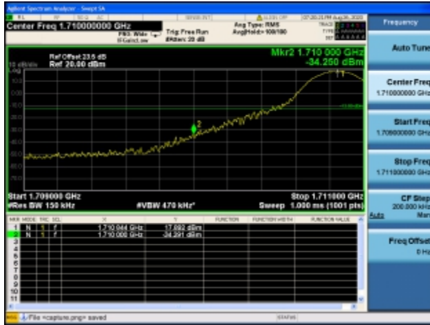
Band4 / 15MHz / High CH / QPSK / 1 RB
