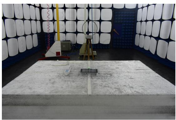
3. Radiated emission (9KHz-30MHz)
