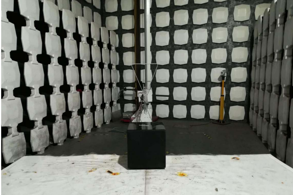
Radiated Spurious Emissions Below 1000MHz
