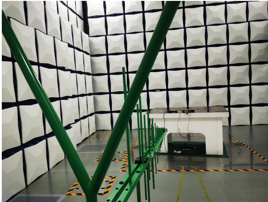
Photograph 3: Set-up photo for Radiated Emissions Below 1GHz
