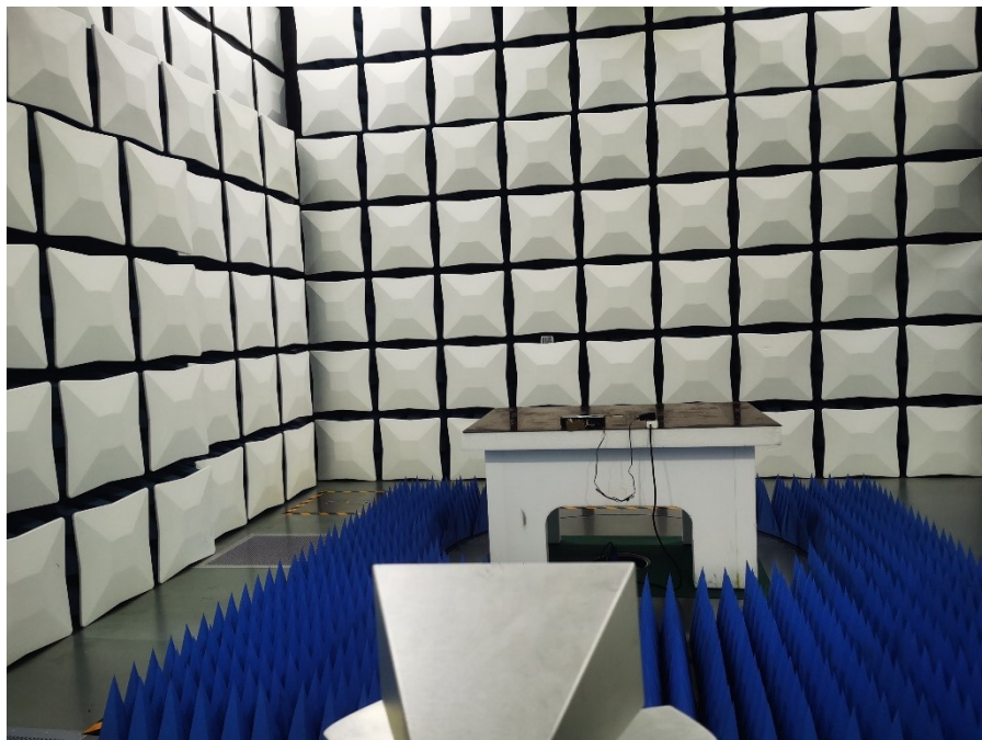
Photograph 4: Set-up photo for Radiated Emissions Above 1GHz
