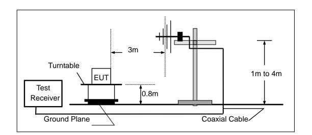
(C) For radiated emissions above 1000MHz
