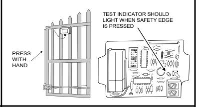
Wire Receiver. Wire receiver obstacle output to obstacle input on operator. Refer to operator and receiver wiring instructions.
