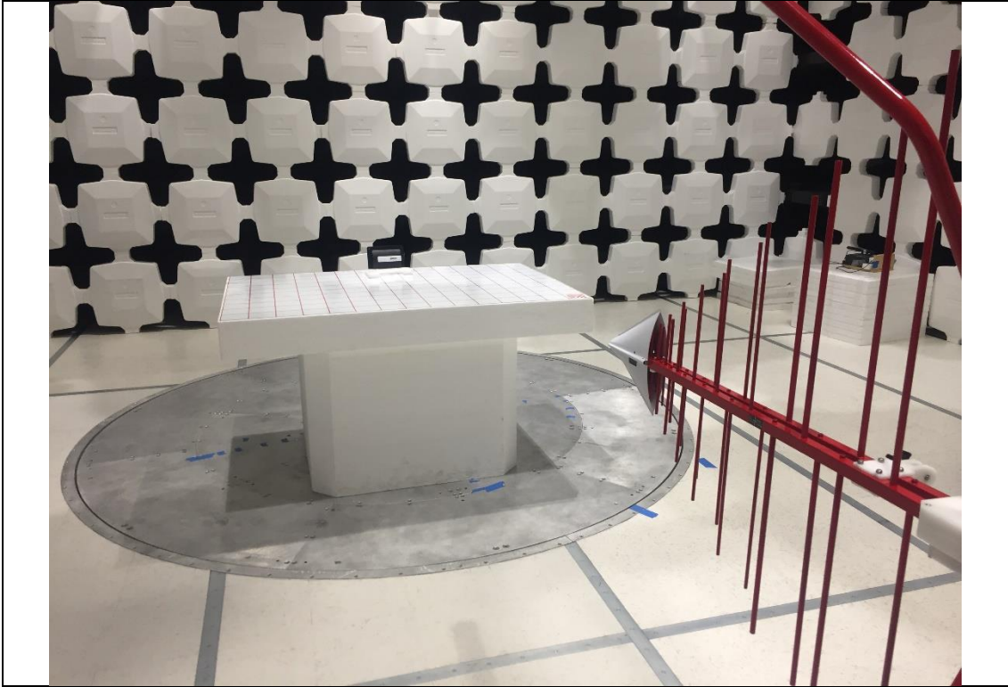
Radiated Emissions Below 1GHz setup – Front
