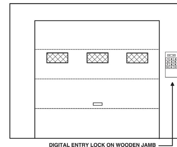
**IF YOU ARE MOUNTING YOUR KEYLESS ENTRY SYSTEM TO ALUMINUM SIDING** you may find it better to substitute carriage bolts for the mounting screws supplied. Bolts should be long enough to reach into the garage, and be secured with lock-washers and nuts. **IF YOU ARE MOUNTING YOUR KEYLESS ENTRY SYSTEM ONTO BRICK, STONE, OR MORTAR**, suitable anchors must be set into the mortar, and the fasteners screwed into these.
