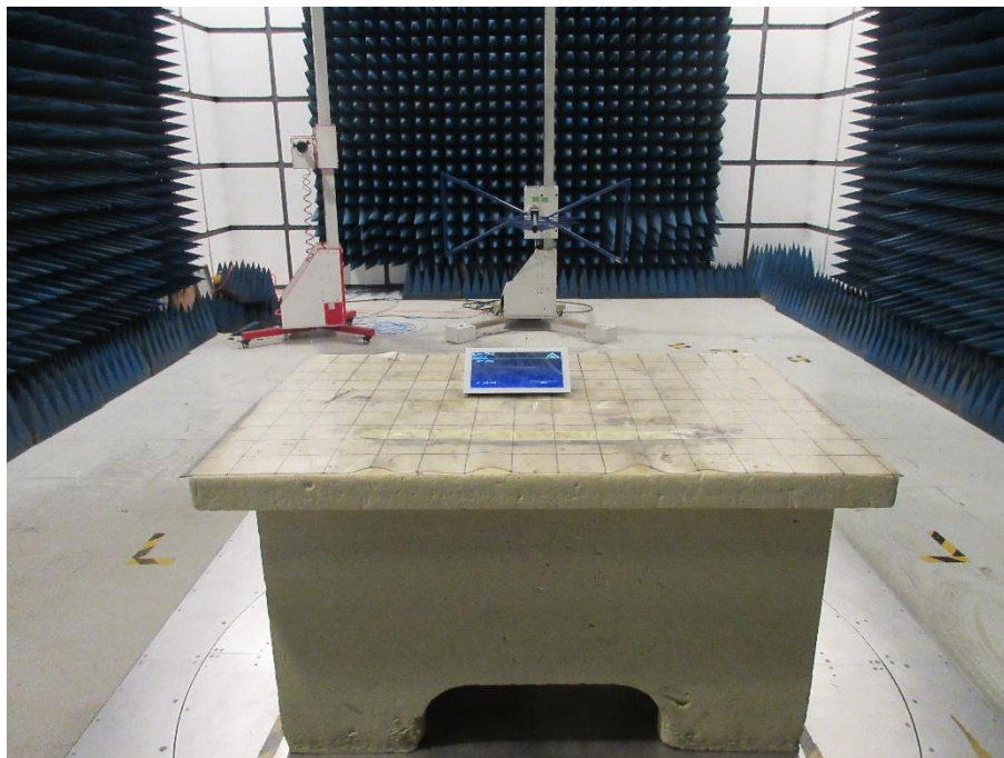
Radiated SPURIOUS EMISSION SET-UP PHOTOS, 30MHz ~ 1GHz
