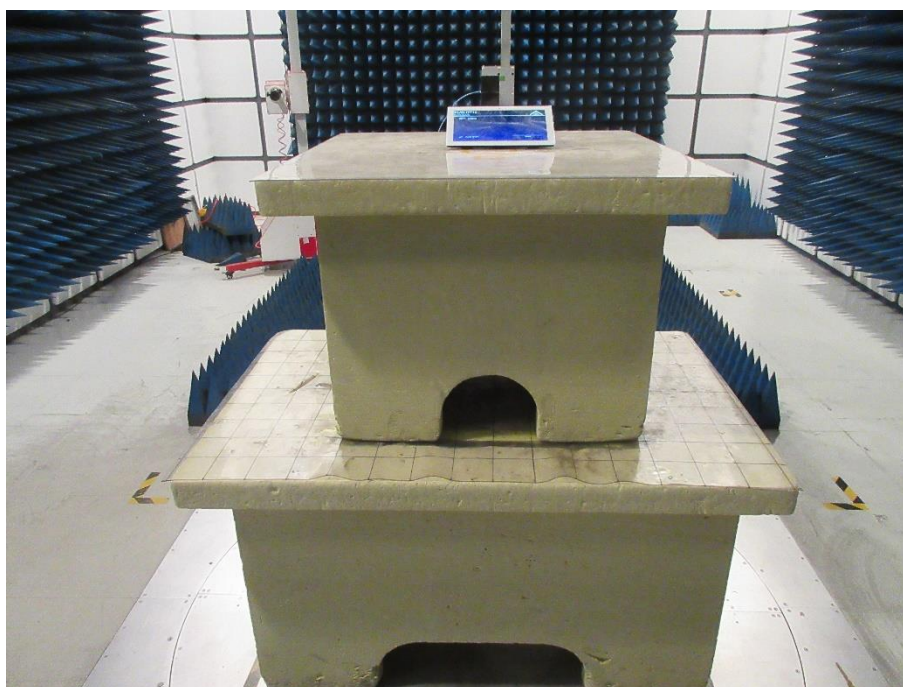
Radiated SPURIOUS EMISSION SET-UP PHOTOS, 1GHz ~ 25GHz
