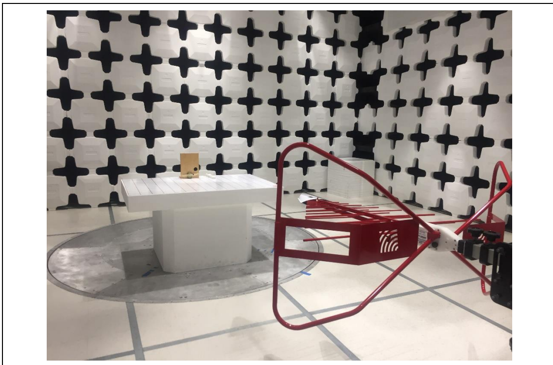
Radiated Emissions Below 1GHz setup – Front
