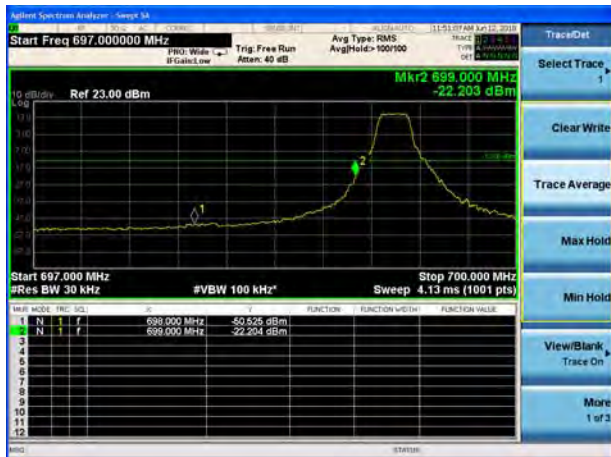
LTE Band 12 16QAM 5MHz CH-Low, 1 RB
