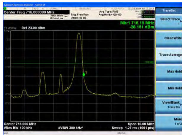
LTE Band 12 16QAM 3MHz CH-High, 1 RB 716MHz~717MHz
