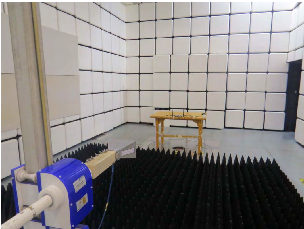
Picture 2: Radiated Spurious Emissions Test setup
