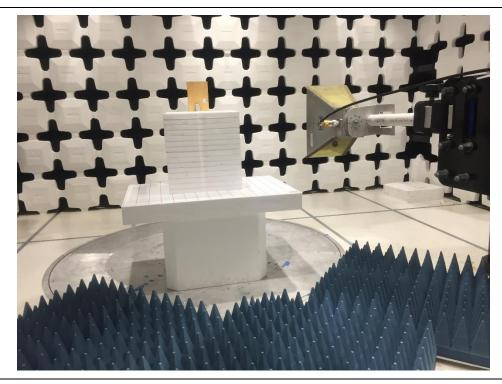
Radiated Emissions Above 1GHz setup – Front
