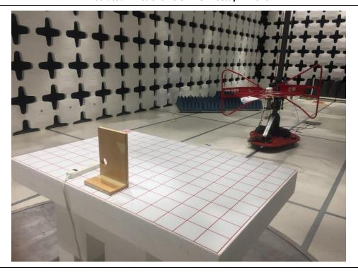
Radiated Emissions Below 1GHz setup – Rear
