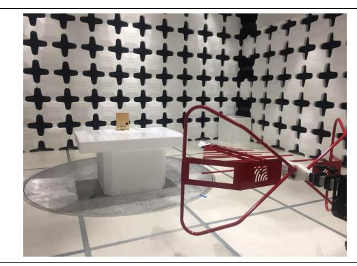
Radiated Emissions Below 1GHz setup - Front
