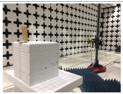
Radiated Emissions Above 1GHz setup – Rear
