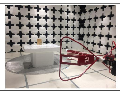
Radiated Emissions Below 1GHz setup - Front
