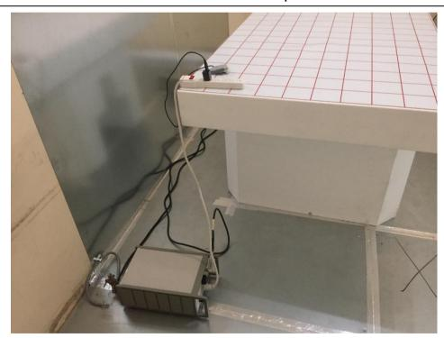
AC Line Conducted Emission setup - Rear
