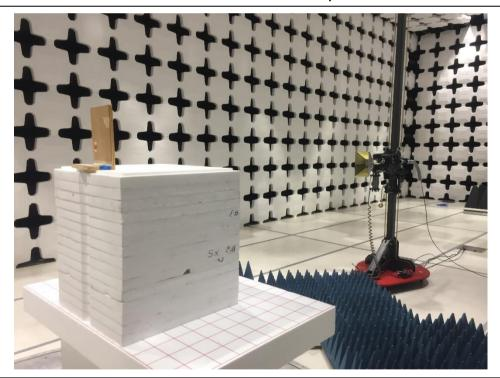
Radiated Emissions Above 1GHz setup - Rear
