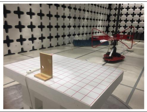
Radiated Emissions Below 1GHz setup - Rear
