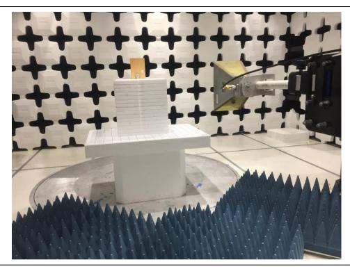
Radiated Emissions Above 1GHz setup - Front
