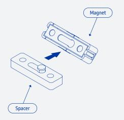
2. Slide spacer forward to lock it onto the magnet.
