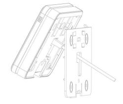
(b) If down the wall, the cord is routed through the channel on rear of Keypad.
