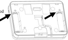
the table stand into the back housing. Then apply pressure to the bottom tabs until the bottom tabs can be inserted into the bottom housing.
