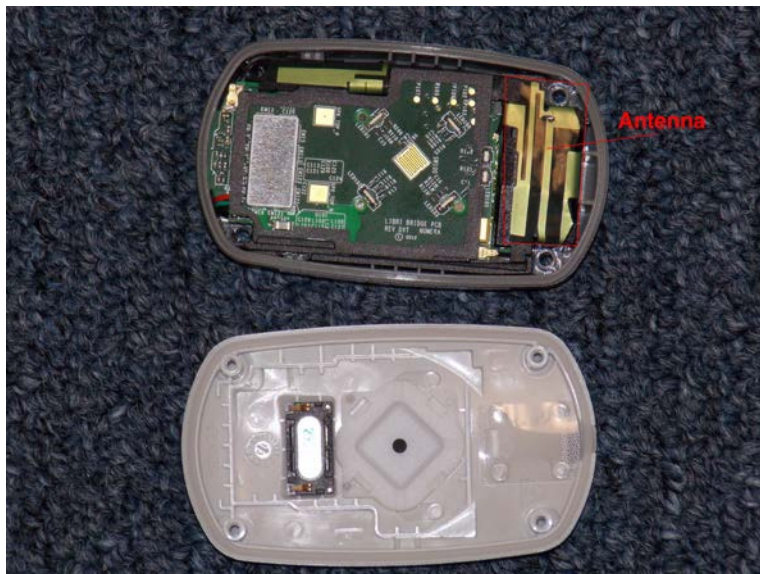
Front Cover Removed
