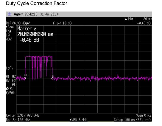
This plot shows all packets of transmissions in 100ms. Total time that packet group is on equals 20 ms (off time with group not measured)
