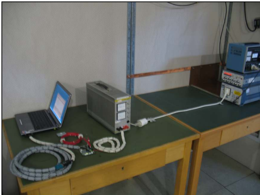
Photo 4: AC Line Conducted Emissions
