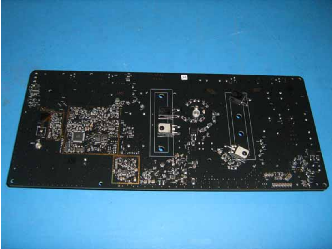
Figure 2: Internal Photo of SM5400 without Plastic Enclosure (Rear Side)
