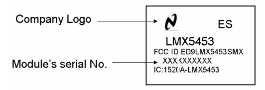
if the module is installed inside another device, then the outside of the device into which the module is installed must displayed a label referring to the enclosed module. This exterior label can use wording such as the following:
