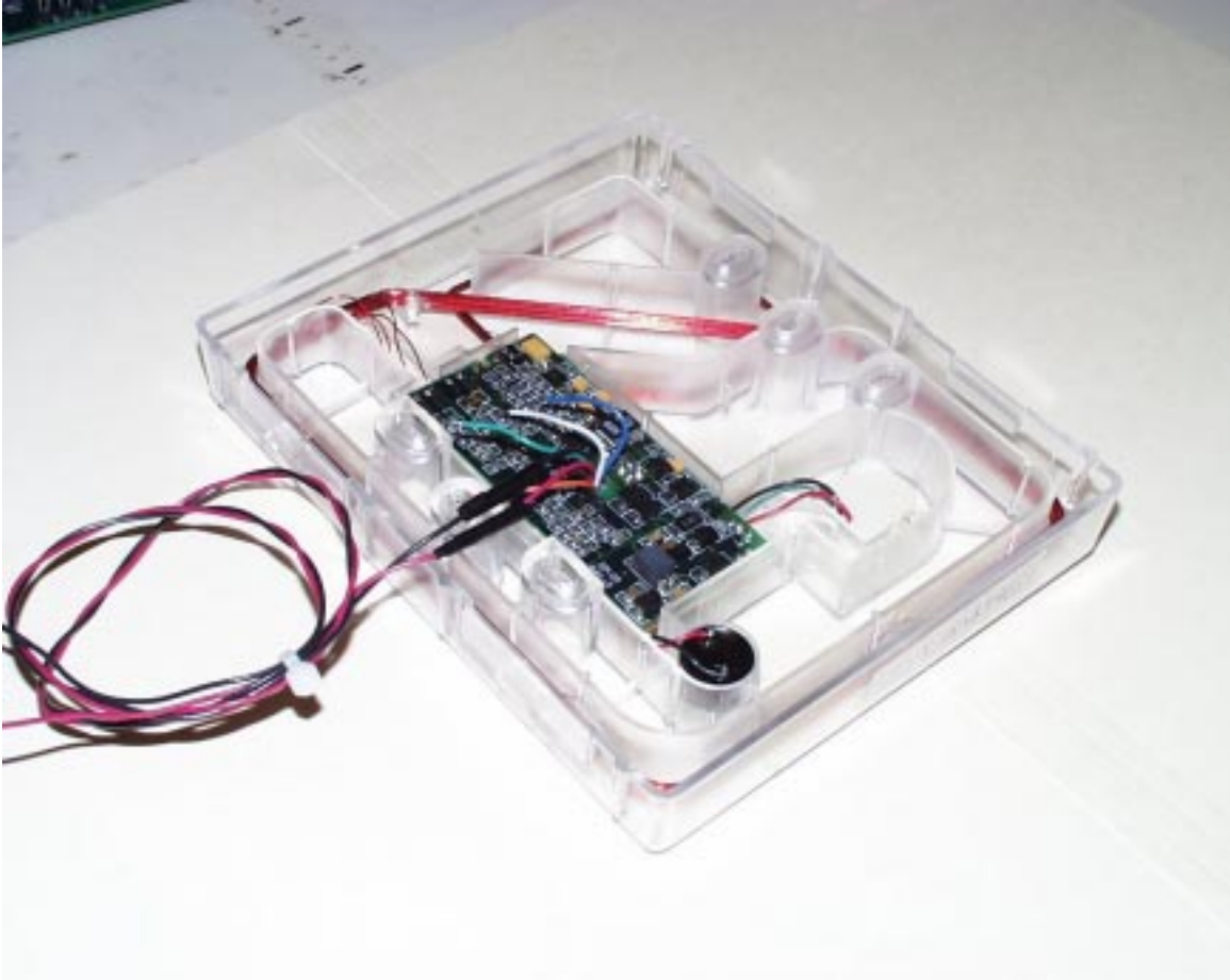
Figure 9.0-2 Internal Photo 2, no potting
